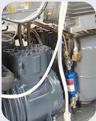
ECOGEL batch freezers are equipped with two parallel refrigeration systems that allow a reduction of 20% of nominal power applied and reduce, as a result, the consumption of energy and water. The emptied cylinder can be kept cold between  $+1^{\circ}\text{C}$  to  $+3^{\circ}\text{C}$ .
